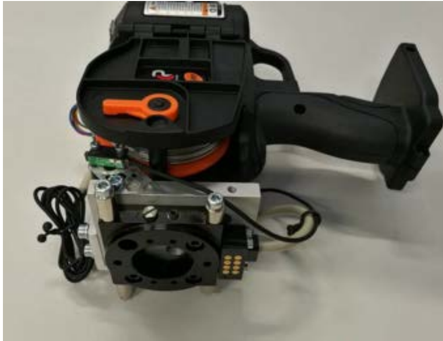
Figure 46 - Tying tool with adapter plate
