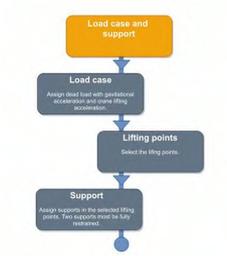
Figure 27, Workflow for assigning load case and support in the Finite Element Model
