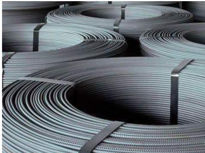
Figure 3 - Coiled reinforcing bars (concrete-mesh, 2016)
