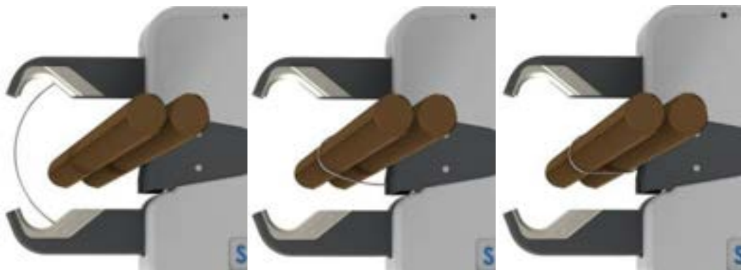
Figure 31 – Illustration of tying process divided in three steps
